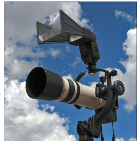
Flash X-tender on Canon 550 flash. Shown with Canon 100-400 lens with F-6 Wimberley flash bracket and Wimberley Sidekick bracket
